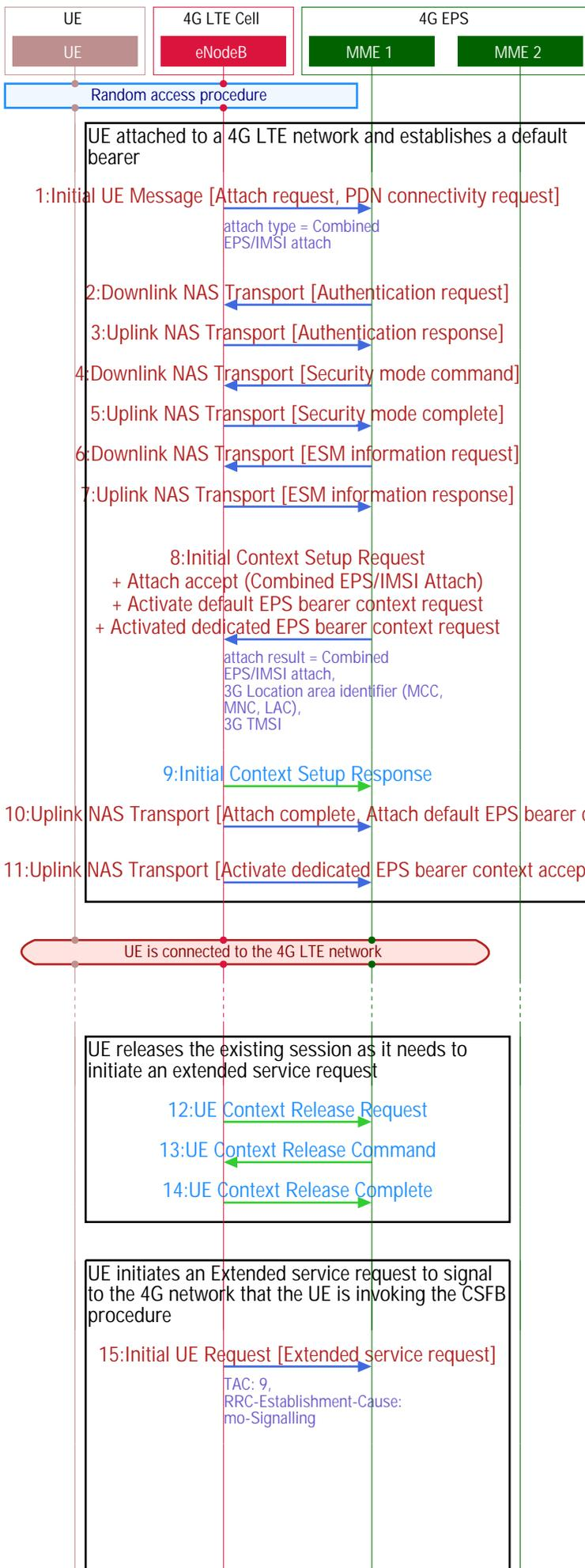
The UE establishes an RRC connection with the LTE eNodeB.
