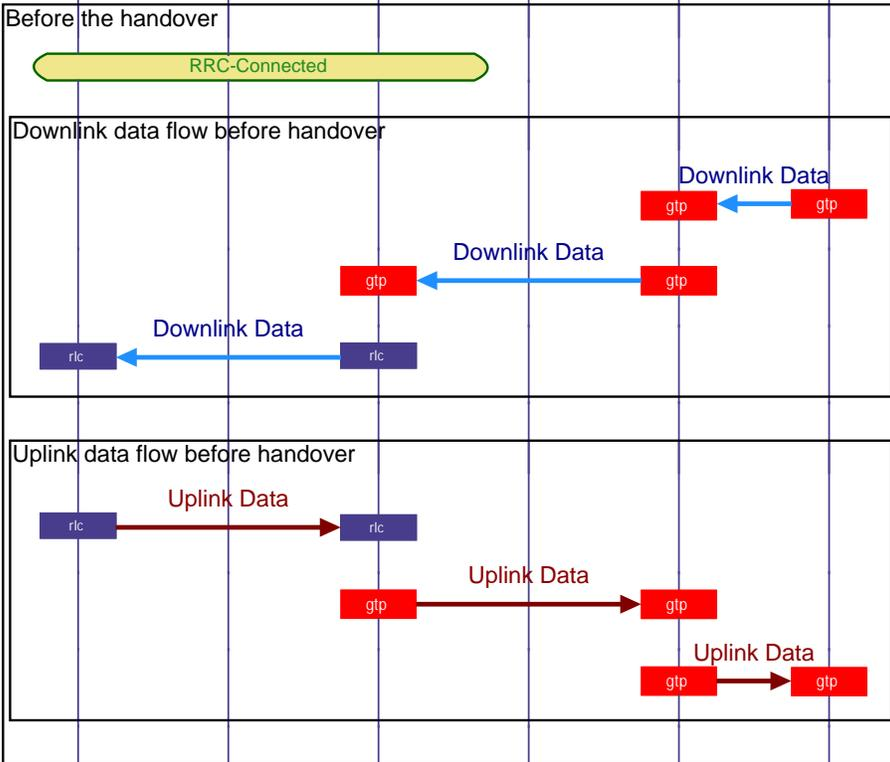
The UE and Source eNodeB are in RRC Connected state.
