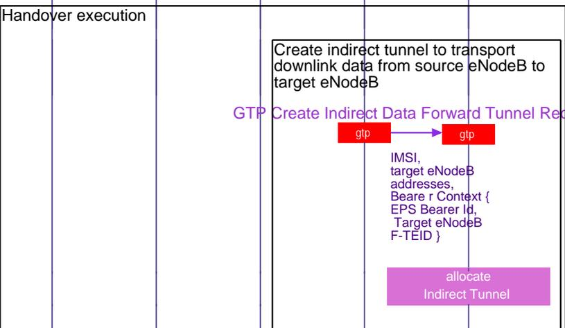
No X2 path exists between the source and target eNodeB, so a tunnel needs to be established between the source and target eNodeBs via the SGW.
