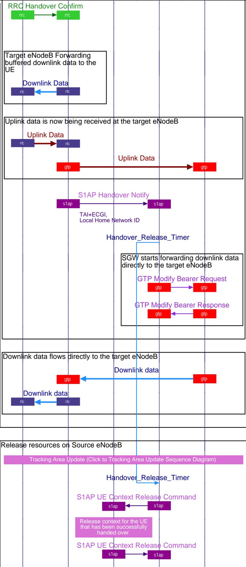
After the UE has successfully synchronized to the target cell, it sends a Handover Confirm message to the target eNodeB. Downlink packets forwarded from the source eNodeB can be sent to the UE. Also, uplink packets can be sent from the UE, which are forwarded to the target Serving GW and on to the PDN GW.
