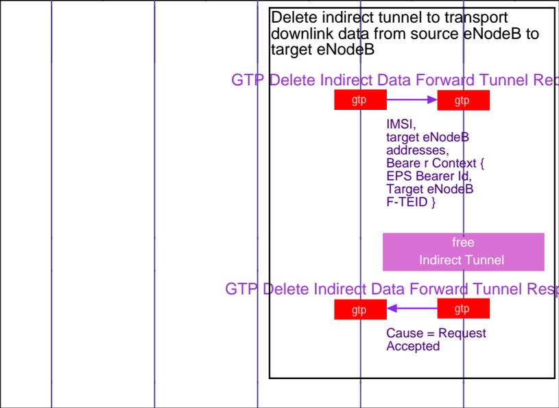
MME requests removal of the indirect tunnel between source and target eNodeBs.
