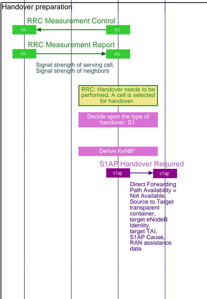
The network sets the measurement thresholds for sending measurement reports.
