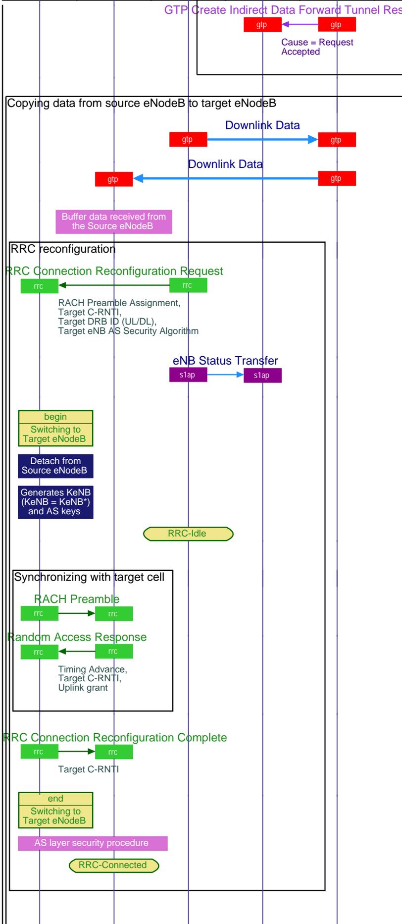
The downlink data is transported from the Source eNodeB to the Target eNodeB via the just established indirect tunnel.
