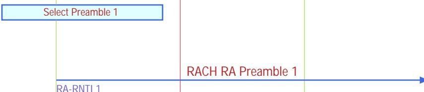
The UE-A randomly selects an RA preamble sequence from the set of sequences available in the cell. The preamble selection is a shift in the Zadoff-Chu code for the cell.
