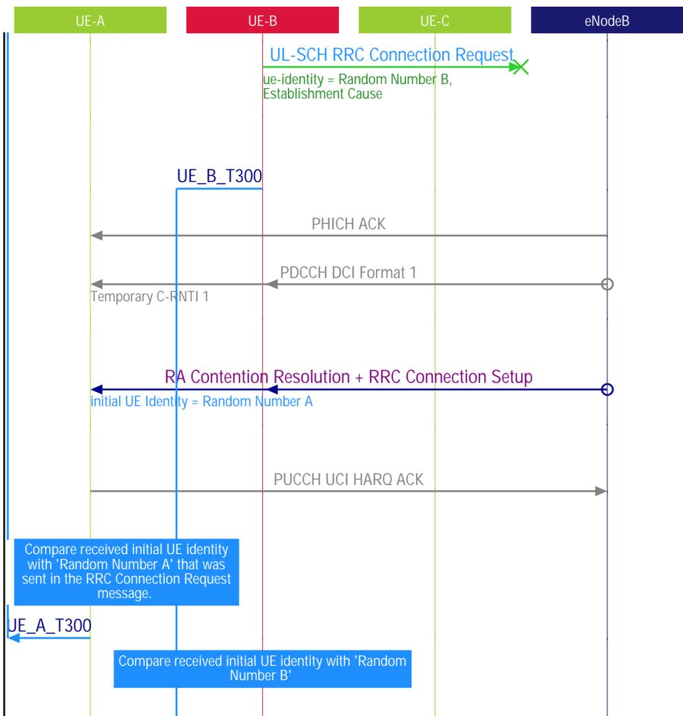
UE-B transmits on the same assignment and collides with the transmission of UE-A. It is likely that its transmission will not be received at the eNodeB as it is transmitting with a timing advance that was not intended for the UE. In this scenario, UE-B's message is lost.
