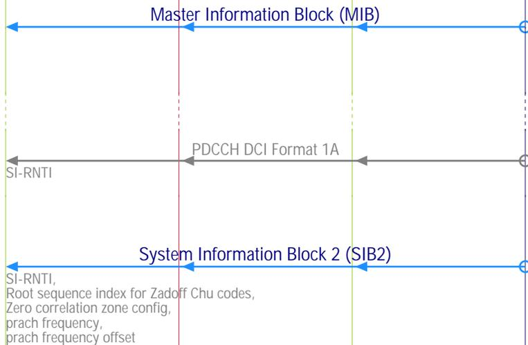
UEs download the MIB from the broadcast channel. This channel contains information about the location of the downlink and uplink carrier configuration.
