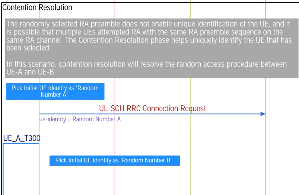
The randomly selected RA preamble does not enable unique identification of the UE, and it is possible that multiple UEs attempted RA with the same RA preamble sequence on the same RA channel. The Contention Resolution phase helps uniquely identify the UE that has been selected.
