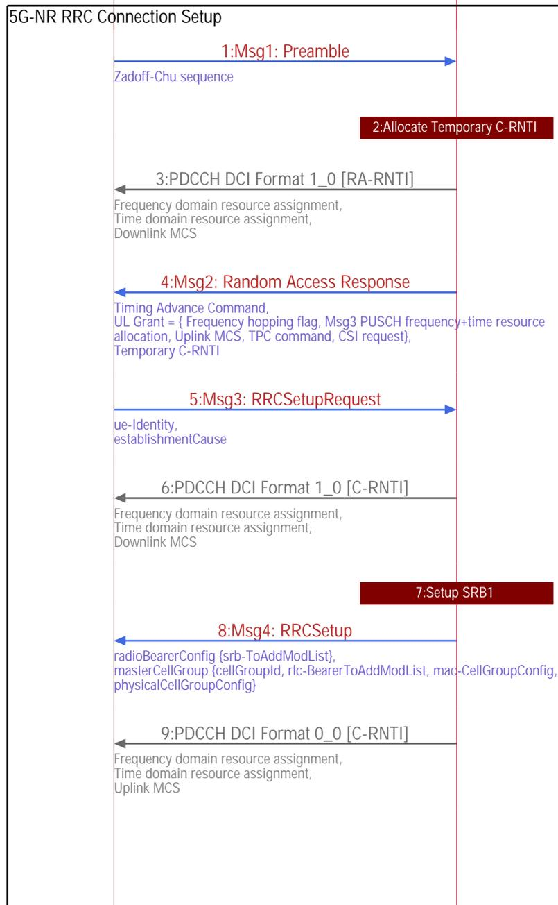
The UE picks a random preamble. The preamble is referenced with the Random Access Preamble Id (RAPID). The preamble transmission is a Zadoff-Chu sequence.
