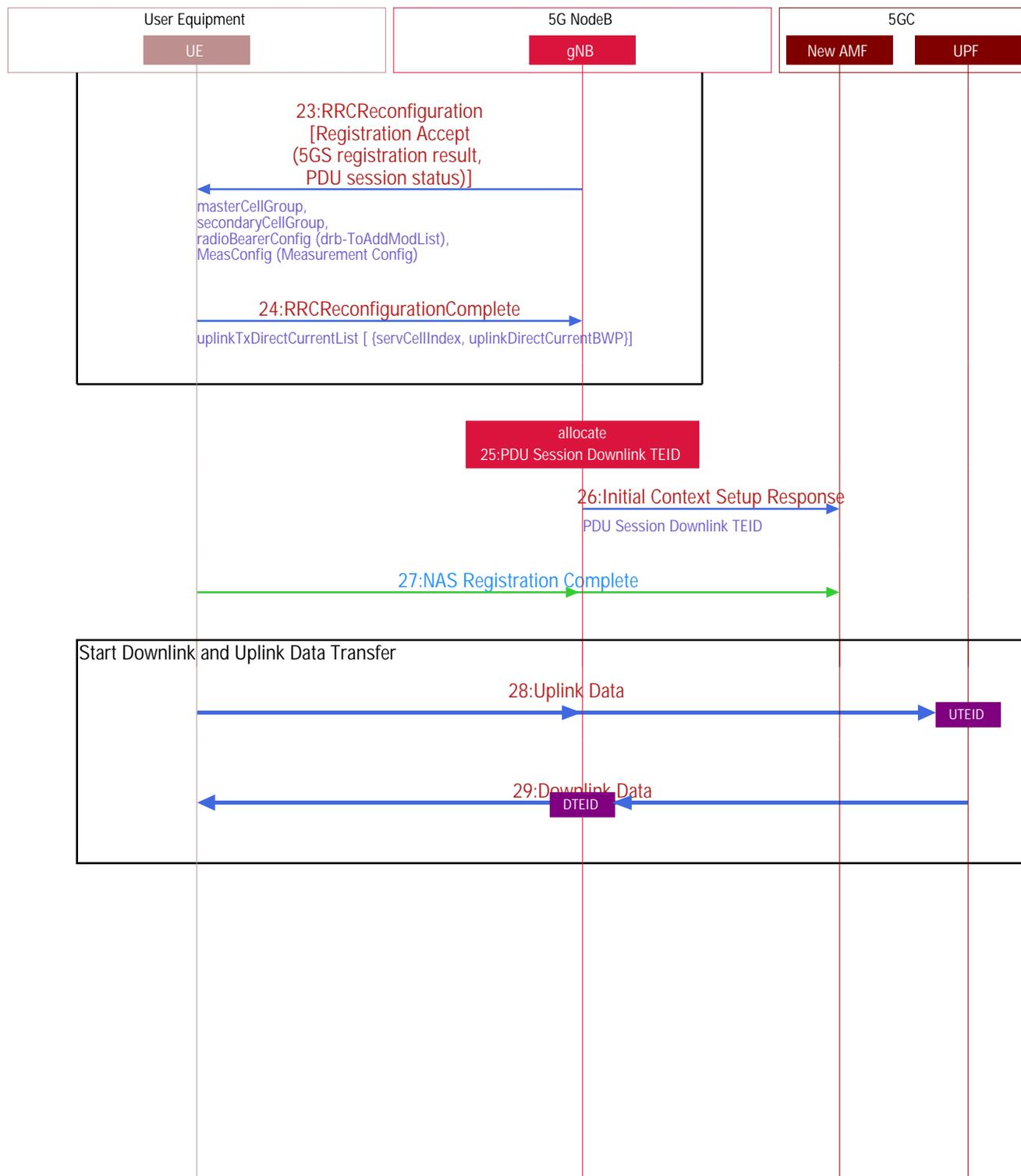
The RRC Reconfiguration message is sent to the UE for setting up radio bearers, setup a secondary cell and initiate UE measurements.
