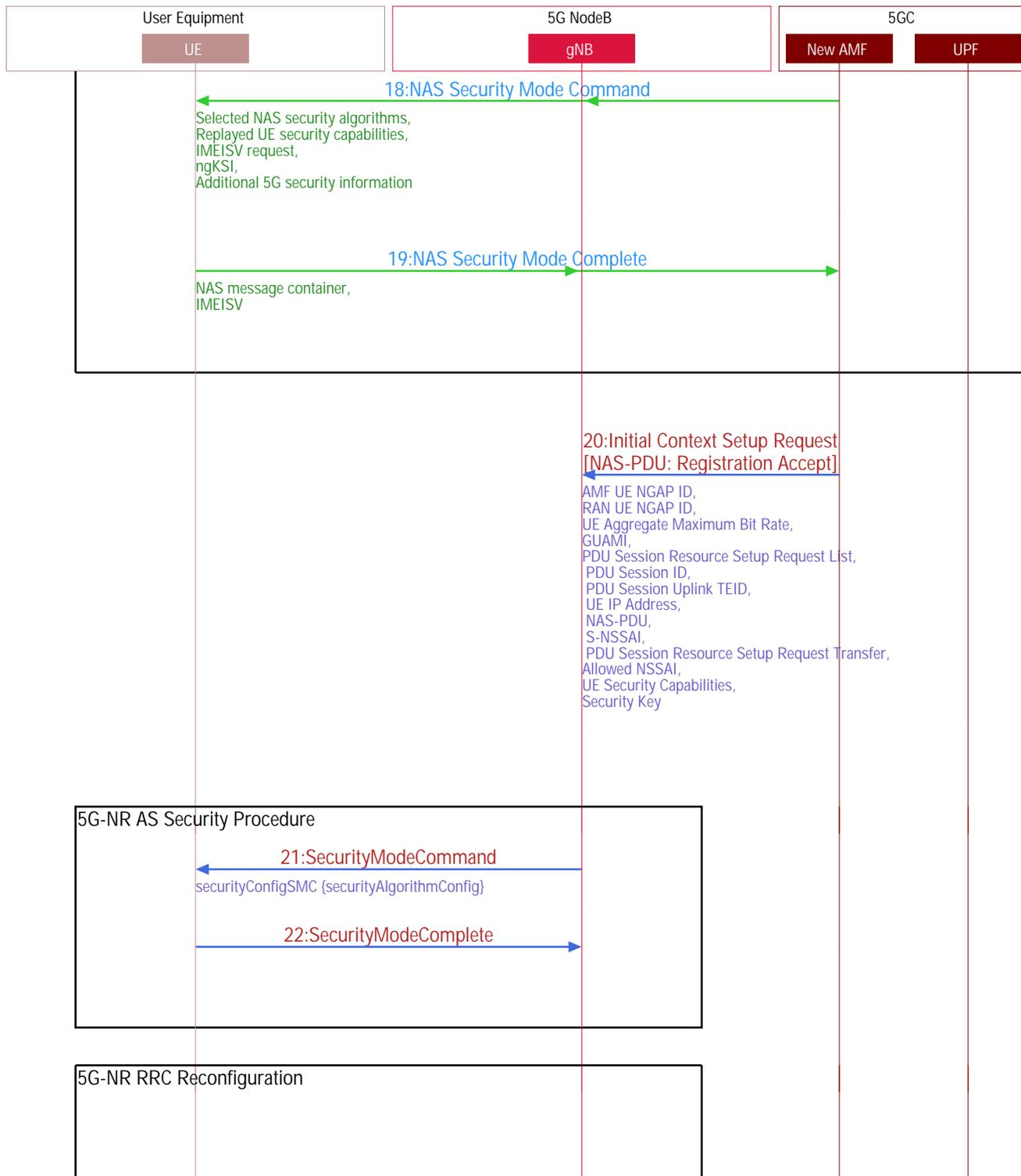
The AMF signals the selected NAS security algorithm to the UE. The AMF also requests the IMEISV from the UE.
