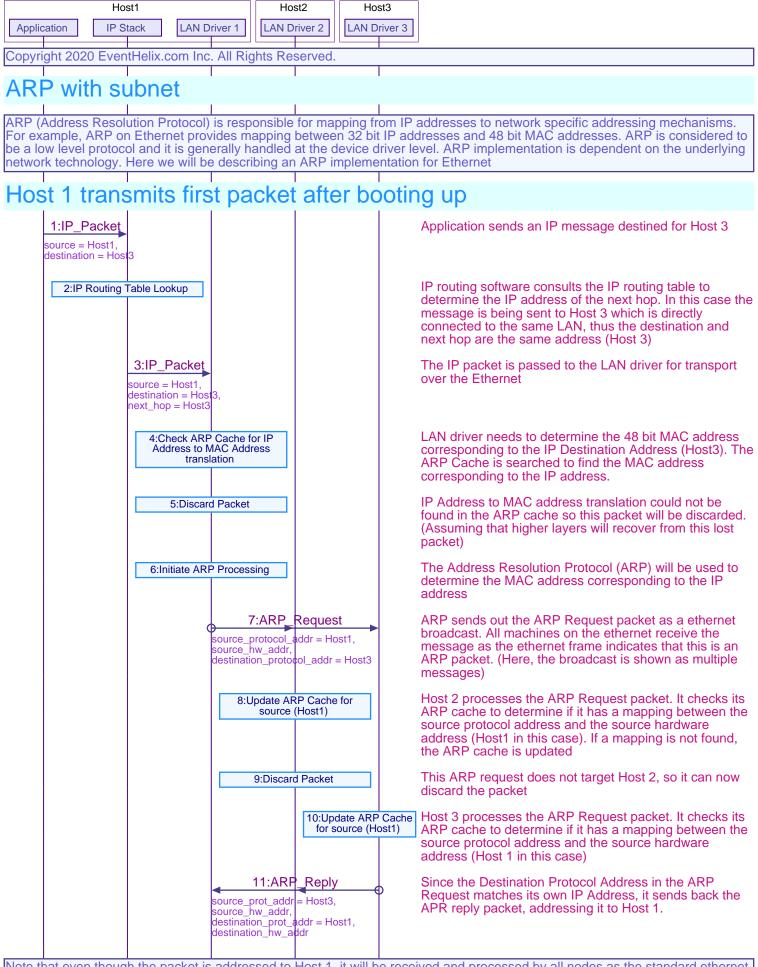
Note that even though the packet is addressed to Host 1, it will be received and processed by all nodes as the standard ethernet frame contains a field specifying that this ethernet frame contains an ARP packet
