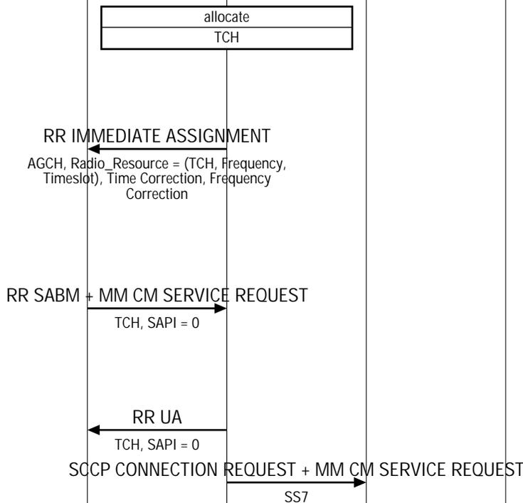
The BSS allocates a Traffic Channel (TCH) to the mobile. The TCH allocation assigns a specifies a frequency and a timeslot on that frequency. After the mobile receives this message, the mobile shall only use the specified resources for communication with the mobile network.
